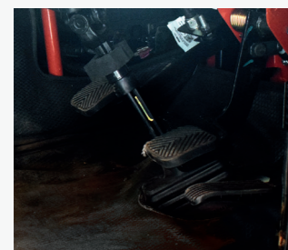
ABC Pedals: Improved Ergonomic pedal positions to reduce fatigue
